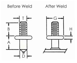
**Aluminum collar studs** are partially threaded studs with a collar separating the weld base and thread. They are available in thread diameters from 1/4" through 1/2".
