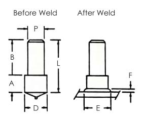
Aluminum SB (Shoulder Base) welding pins are plain, unthreaded fasteners with a weld base diameter greater than the extension diameter. Available with weld base diameters from 1/4" through 1/2"; extension diameters, 1/8' through 3/8".
